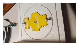
One more hurdle had to be cleared with the latest version of the Gilbertson PVC box. The new ones now have a PVC board as the roof, which lasts much longer than wood, but also is much denser and harder to insert a screw. The solution was to install a moly in the hole, screw through the scented tree and into the moly, problem solved.
