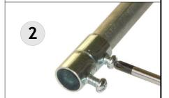
Attach 1/2" EMT coupler to end of conduit. Tighten upper screw against conduit. Install longer screw in bottom but do not tighten.
